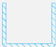
A101 - Frame + sash reinforcement U 24x28x24x1.5 A102 - Frame + sash reinforcement U 24x28x24x2
